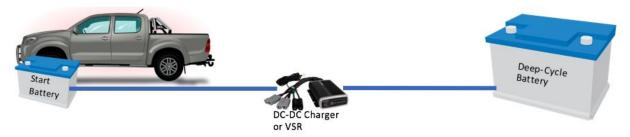
If you've heard of things like a DC-DC charger or VSR (Voltage Sensitive Relay) these are pieces of equipment that go between your car's start battery and the deep-cycle battery, this is to make sure that the battery is charged enough, but not too much and to make sure that the start battery never gets drained.
